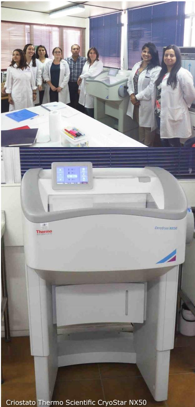
Criostato Thermo Scientific CryoStar NX50
